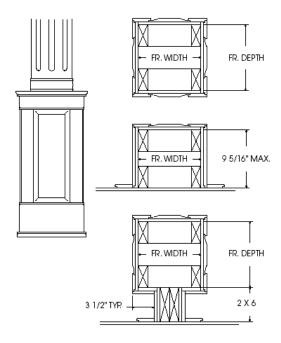
To create columns or pilasters that will exactly fit the Raised Panel System components, follow these guidelines.
