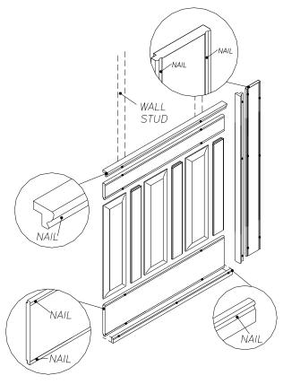
Nail in the grooves of the system. Never on the face of the panels or stiles.
